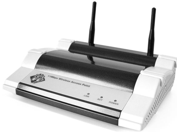
Figure 1.12 GigaFast 802.11b wireless access point. (Courtesy of GigaFast Ethernet USA)
