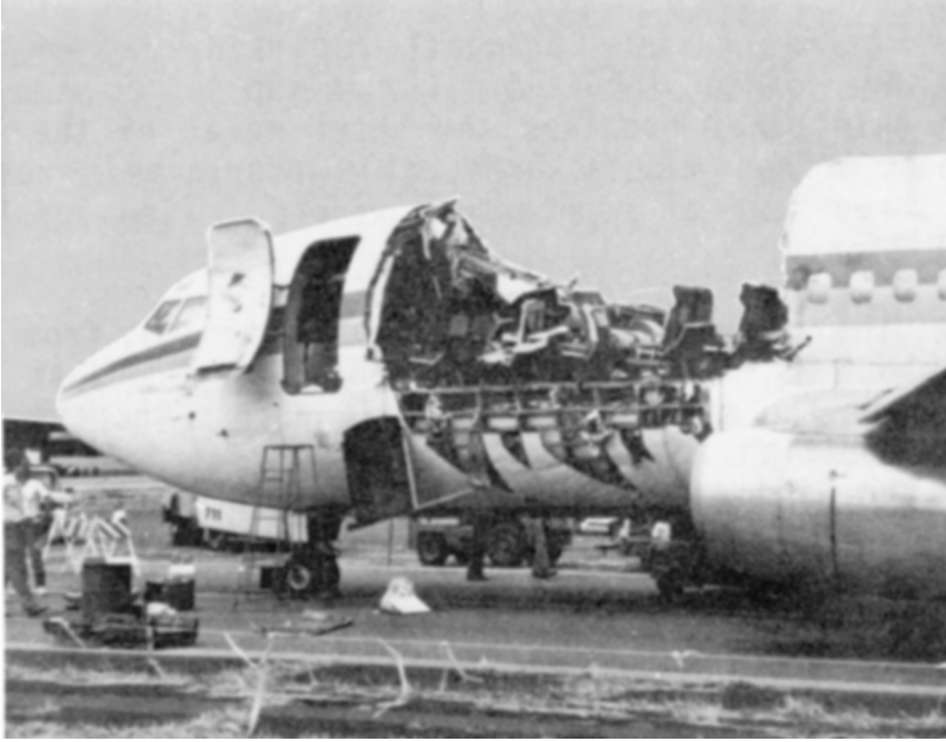
Fig. 1-5. General view showing the damage sustained by the Aloha Airlines 737. (From NTSB, 10.)
