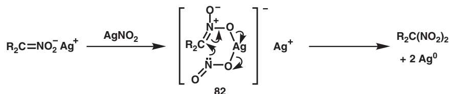
Figure 1.34 Proposed mechanism for oxidative nitration (ref. 105)
