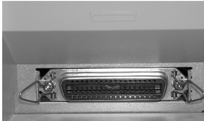
FIGURE 1.62 A Centronics connector
