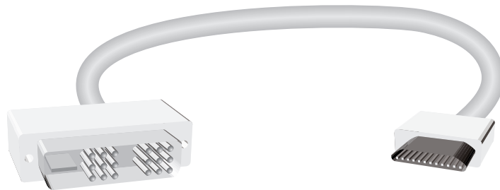
FIGURE 1.45 Types of DVI connector
