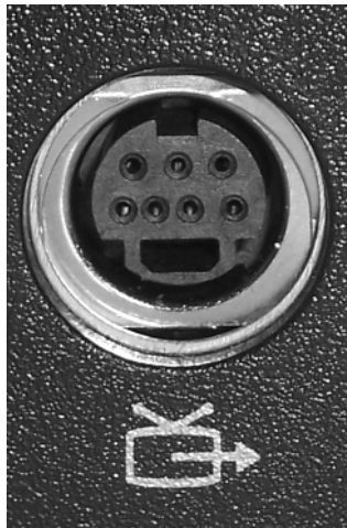
FIGURE 1.47 A 7-pin S-video port
