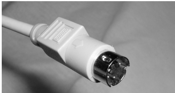
FIGURE 1.72 A PS/2 keyboard cable
