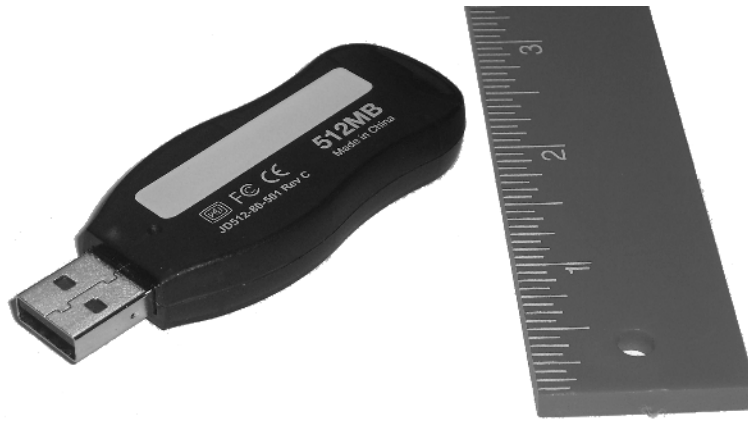
FIGURE 1.34 A USB thumb drive
