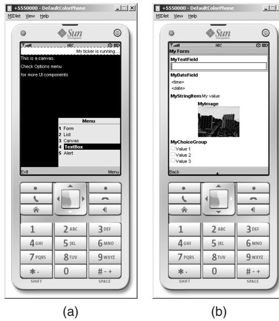
**Figure 2.5** UIExampleMIDlet application running on the WTK emulator: a) the MenuCanvas and b) the Form
