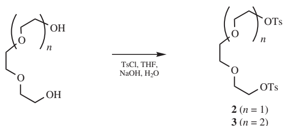
Figure 1.4 Syntheses of triethyleneglycol ditosylate ( 2 ) and tetraethyleneglycol ditosylate ( 3 )
