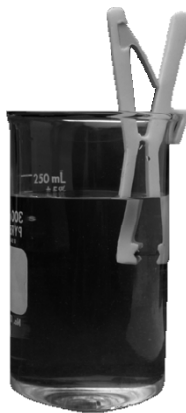
Figure 1.6. Compliant die grippers used to hold a die during process in several different harsh chemicals.
