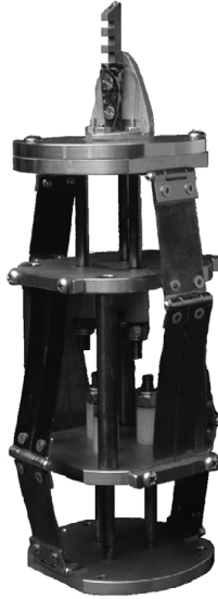
Figure 1.7. Compliant constant-force robot end effector.
