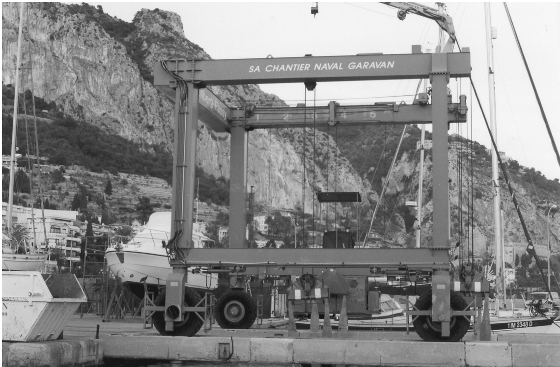
Figure 1.23 Travel lift frame for launching and retrieving pleasure boats.
