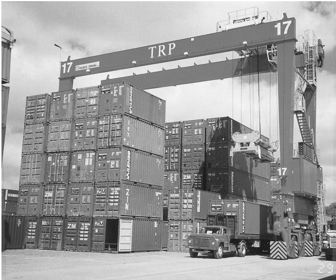
Figure 1.14 Containers stacked in storage area by gantry crane.
