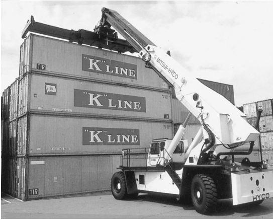
Figure 1.15 Containers stacked by high-reach stacker with telescopic boom.
