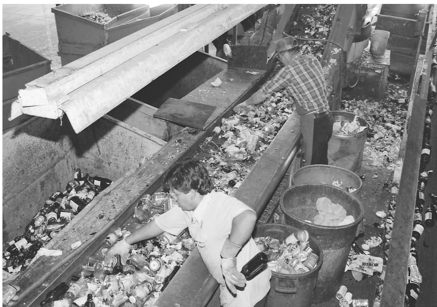
Figure 5-16 Typical sorting line for manual separation of waste components.
