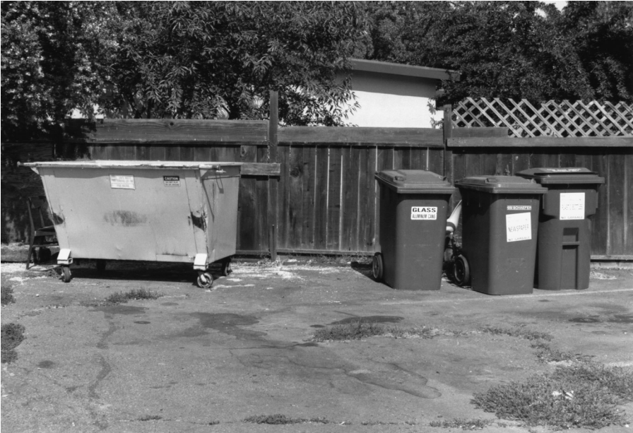
Figure 5-4 Typical examples of large containers used for low- and medium-rise apartments (note separate containers for recyclable materials).
