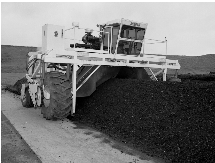
Figure 5-21 View of machine used to aerate compost placed in windrows.
