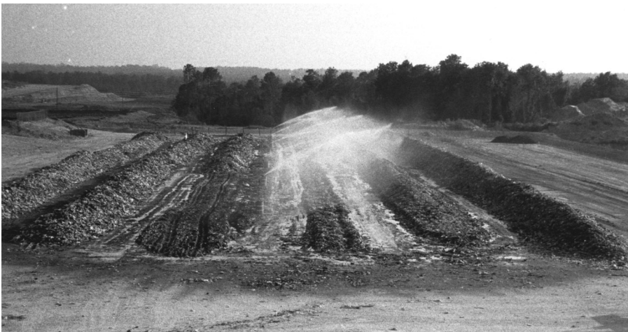
Figure 5-20 Overview of windrow composting operation.
