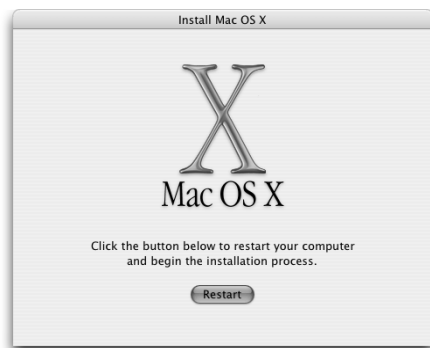
Figure 1-2: The Restart button in the Install Mac OS X program restarts the computer with the Mac OS X Install CD to begin installation.
