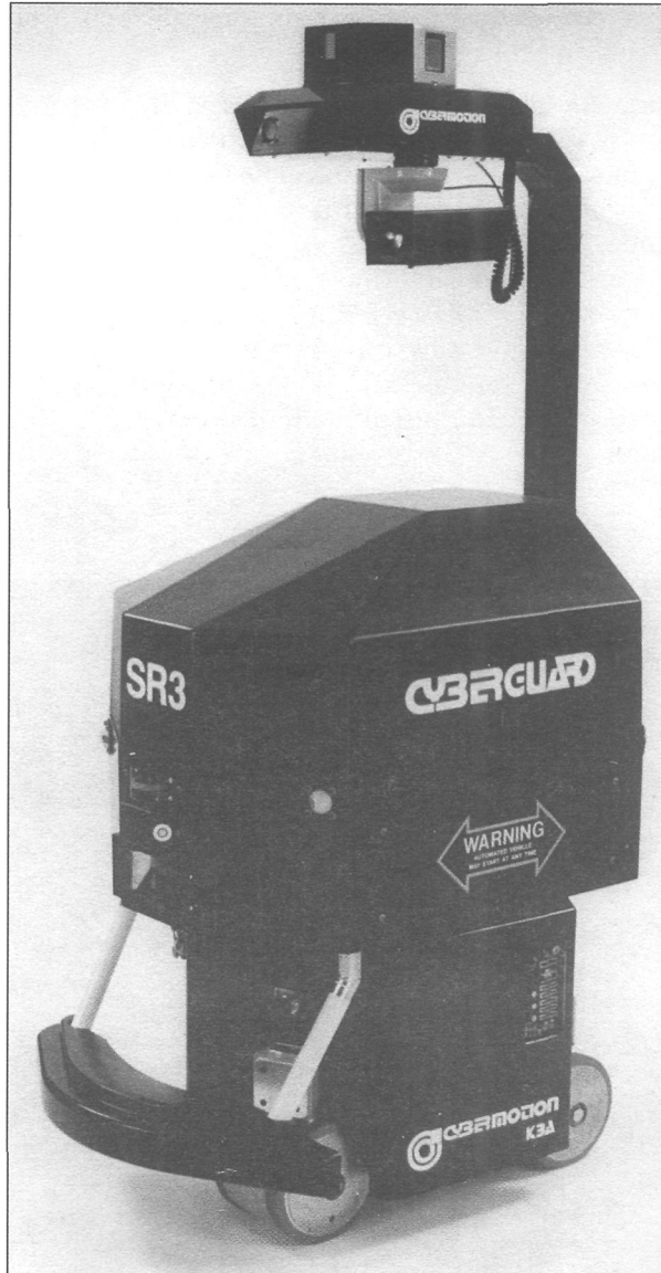
Figure 1.2. The SR 3 Cyberguard Autonomous Robot. Used by permission of Cybermotion, Inc.
