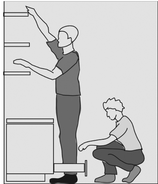
Figure 1-5 Shelves must be within the reach of most users. Drawers and files need additional space in front for the user.
