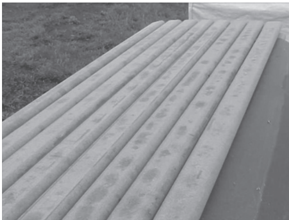
Figure 1.36 Black-colored metabolic products of Gonatobotryum and Epicoccum on the surface of composite handrails.
