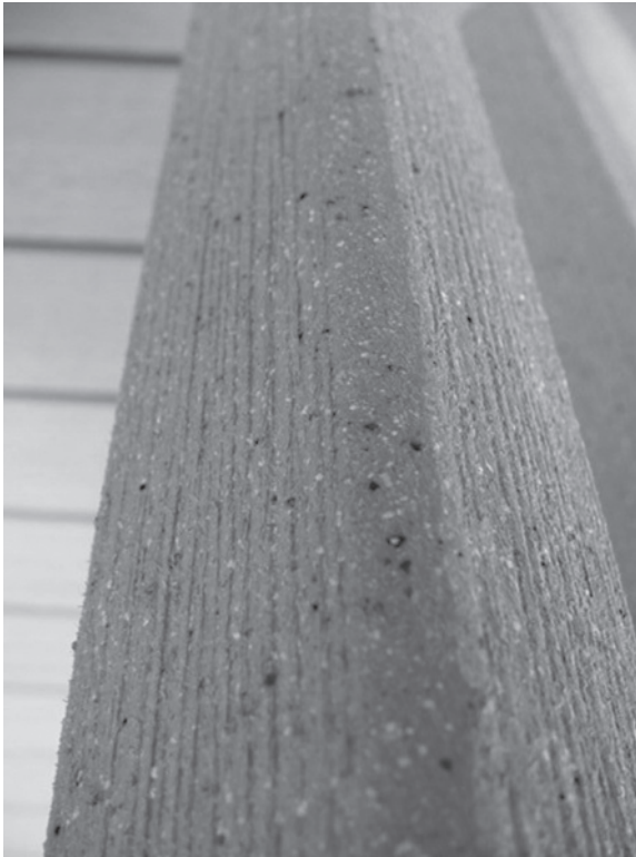
Figure 1.34 Black mold on a WPC material.
