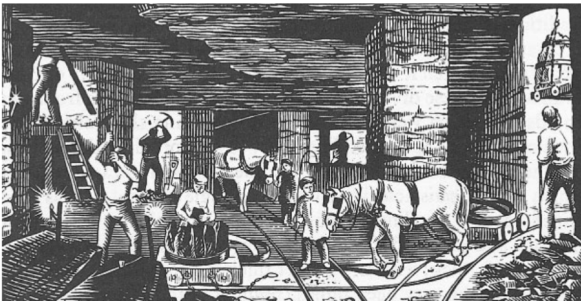
Figure 1-9 Bradley coal mine, Staffordshire. In the early nineteenth century, women carried coal in wicker baskets up 100-foot-tall ladders. Trucks were hauled by women and children who could work in passages too low even for pit ponies. Miners worked in poor ventilation by handpick and crowbar, blasting without a safety fuse until its invention in 1831.
