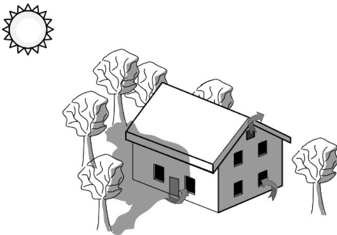
Figure 1-12 Shading and ventilation. Building orientation and landscaping create shade, while window locations aid ventilation.
