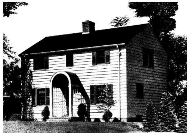
Figure 1-13 Design for temperate climate. This small 1930s house faces the sun, with shade trees sheltering its east and west sides. When the weather becomes colder and leaves fall, more sunlight warms and illuminates the building's interior.
