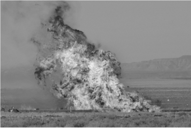
Figure 1.2 Example of a large 23-m diameter LNG pool fire on water (Sandia, 2009).
