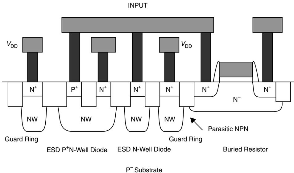
**Figure 1.5** Example of parasitic element parallel to ESD network
