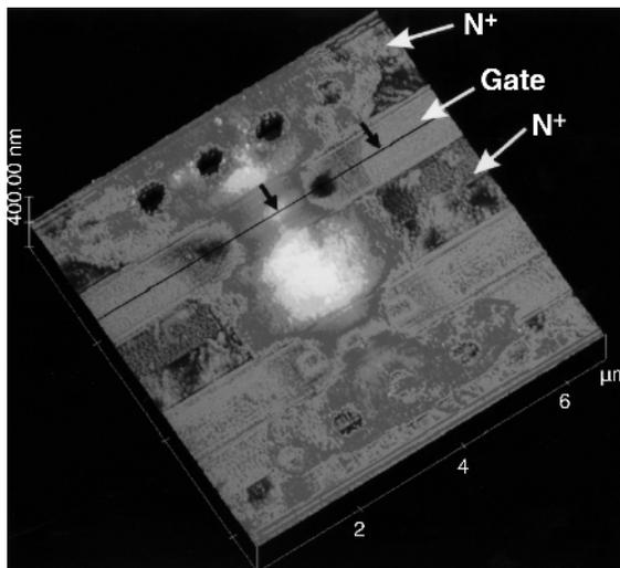
**Figure 1.8** ESD failure between the top MOSFET drain and lower MOSFET source
