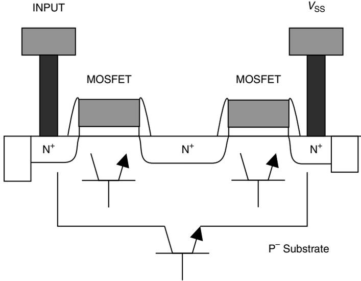
**Figure 1.7** Example of parasitic element in a cascade MOSFET circuit
