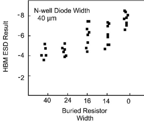
**Figure 1.6** ESD results of parasitic element parallel to ESD network
