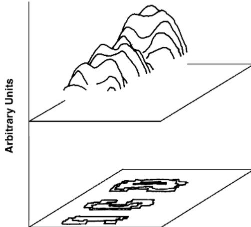
**Figure 1.1** Emission microscope tool photon map of a  $p^+$  diode
