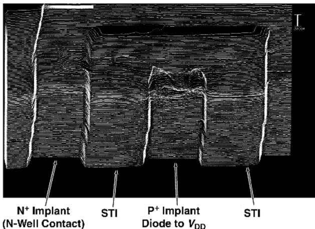
**Figure 1.2** Kelvin probe force microscope topography image of  $p^+$  diode
