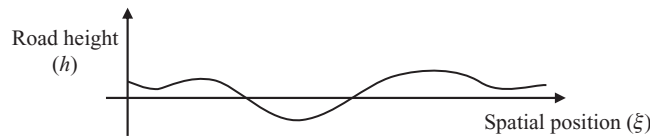
Figure 1.8 An example of a signal where time is not the natural independent variable
