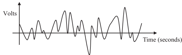
Figure 1.6 A typical continuous signal from a transducer output
