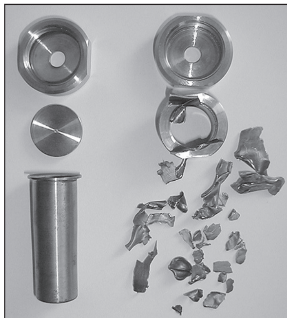
Figure 1.18 Steel sleeves used in Koenen tests: before (left) and after the test (right). Courtesy of Prof. Dr Thomas Klapötke, Ludwig-Maximilians University, Munich, Germany
