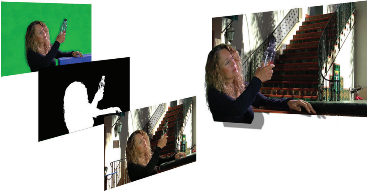
Figure 1.12 The green screen traveling matte production sequence
