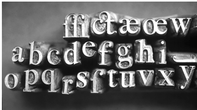
Actual Bodoni punches. Carved punches were driven into other pieces of metal called matrices. Molten metal was then poured into these matrices, making the actual type. Courtesy of Sumner Stone.
