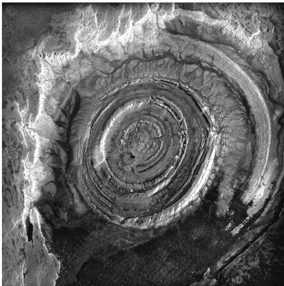
Figure 1.14 X-band Synthetic aperture radar (SAR) image of the Richat geological structure in Mauretania collected by the Italian satellite COSMO-Skymed 1 on 8 October 2007. The structure is about 60 km in width. COSMO-Skymed (COntellation of small Satellites for Mediterranean basin Observation) plans to have five satellites in orbit eventually. The third was launched in October, 2008. ( http://www.telespazio.it/GalleryMatera.html ). COSMO-SkyMed Product © ASI-Agencia Spaziale Italiana (YEAR) – All Rights Reserved.
