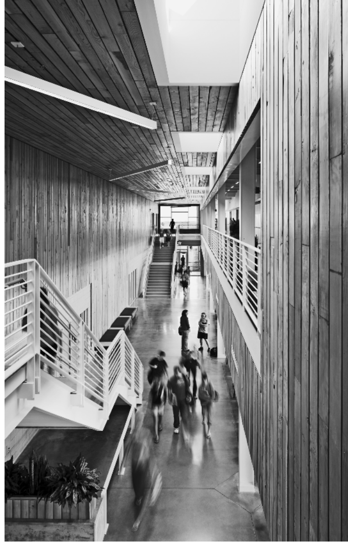
Kiowa County Schools—Main Street. The primary circulation hallway in the school is called “Main Street.” The wide, open hallway is a gathering space for students. It is daylit and clad with wood that came from salvaged cypress trees downed during Hurricane Katrina. Firm: BNIM. PHOTO: © ASSASSI
