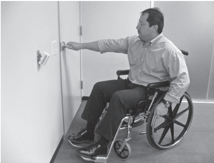
Figure 1.14: This door has plenty of room for a person in a wheelchair to reach the door handle and open the door.
