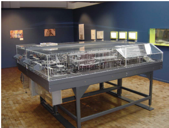
FIGURE 1.6 Replica of the Z1 computer in the German Museum of Technology
