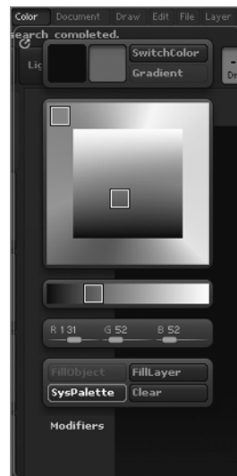
Figure 1.5 The numbers in the R (red), G (green), and B (blue) fields indicate the values for the red, green, and blue channels.
