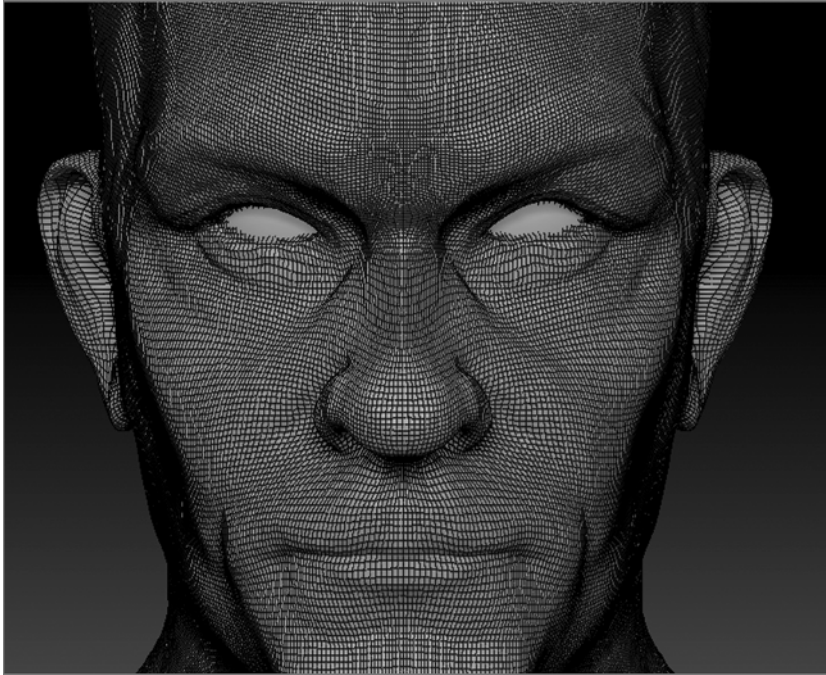
Figure 1.8 A high-resolution model in ZBrush. The lines on the surface show how the model consists of thousands of square polygons.
