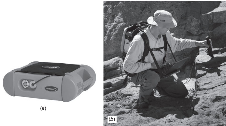
Figure 1.22 ASD, Inc. FieldSpec Spectroradiometer: (a) the instrument; (b) instrument shown in field operation. (Courtesy ASD, Inc.)
