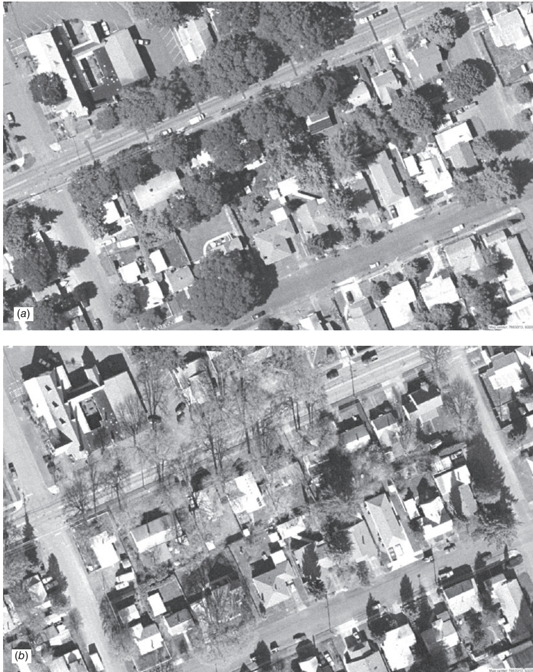
Figure 1.32 Comparison of leaf-on photography with leaf-off photography. Gladstone, OR. (a) Leaf-on photograph exposed in summer. (b) Leaf-off photograph exposed in spring. Scale 1:1,500. (Courtesy Oregon Metro.)
