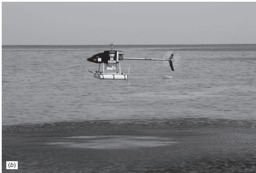
Figure 1.24 Uninhabited aerial vehicles (UAVs) used for environmental applications of remote sensing. (a) NASA's Ikhana UAV, with imaging sensor in pod under left wing. (Photo courtesy NASA Dryden Flight Research Center and Jim Ross.) (b) A vertical takeoff UAV mapping seagrass and coral reef environments in Florida. (Photo courtesy Rick Holasek and NovaSol.)
