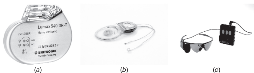
Figure 1.6 Commercial wearable devices: (a) Biotronik defibrillator [Copyright © Biotronik, Inc. (Biotronik, 2012)]; (b) Nucleus Freedom Cochlear Implant [Image courtesy of Cochlear Americas (Nucleus Freedom, 2010)]; (c) Second Sight Argus II Retinal Prosthesis [Copyright © 2013 Second Sight Medical Products, Inc. (Second Sight, 2012)].
