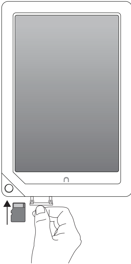
Figure 1-8: Insert a microSDHC card in the slot on the bottom of the device; shown here is the NOOK HD+.
