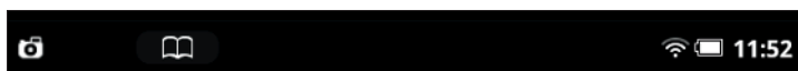
Figure 1-16: This status bar shows, from left to right, a small icon of a camera (because I captured a screen). There's an open book to allow quick access to a recent read. Icons on the far right show the Wi-Fi connection, battery life, and current time.
