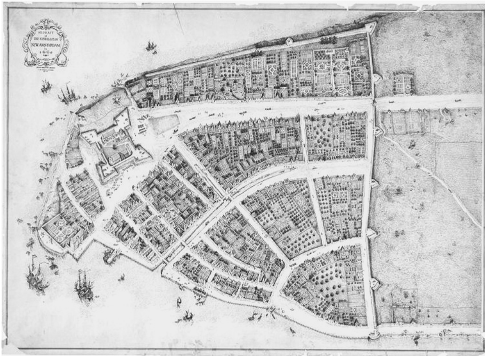
1.7 Plan of New Amsterdam (1660). In nearly twenty years as governor, Peter Stuyvesant turned New Amsterdam's jumbled lanes into a gridded pattern that suggested the influence of both the Three Canals plan and baroque planning sensibilities. Courtesy of I. N. Phelps Stokes Collection, Miriam & Ira D. Wallach Division of Art, Prints and Photographs, the New York Public Library, Astor, Lenox & Tilden Foundations
