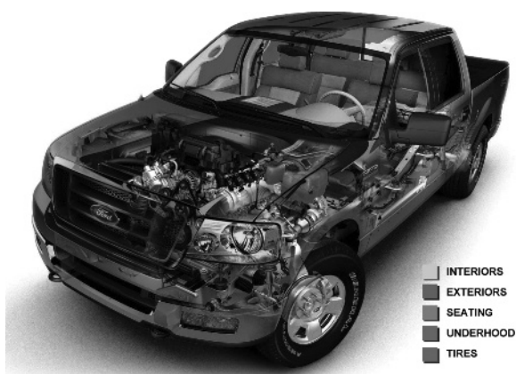
Fig. 4. Overview of Automotive systems using plastics and composites (courtesy of John Jaranson, Ford Motor Company).
