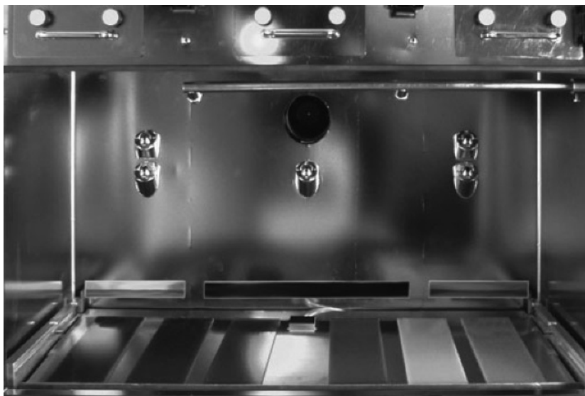
Fig. 5. Interior of a flat-bed xenon-arc weathering instrument. Photo courtesy of Atlas Material Testing Technology LLC.
