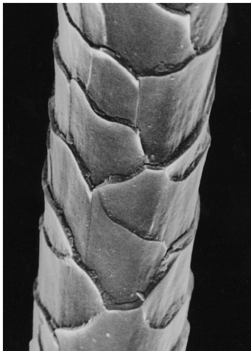
Fig. 2. Scanning electron micrograph of merino fiber, showing overlapping cuticle cells.
