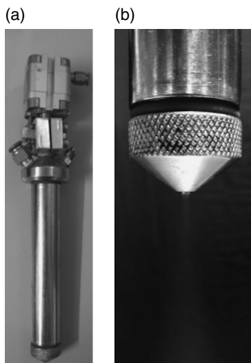
Figure 1.6 (a) Two-fluid nozzle; (b) Spray emerging from two-fluid nozzle.
