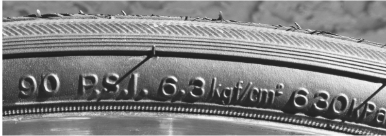
Figure 1.13 Bicycle tire pressure expressed in three different unit systems to meet different consumer preferences within a global market. (Photo courtesy of Richard Figliola.)
