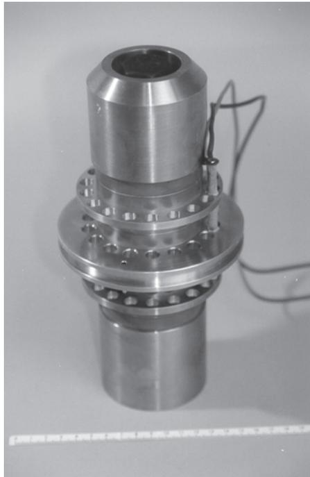
**Figure 1.2** The piezoelectric sandwich transducer.
