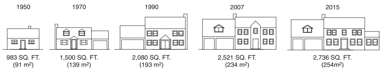
Figure 1-2 The average new home in the United States has grown in size over time—despite the fact that family size has grown smaller. However, larger is not necessarily better, and well-planned spaces need not be excessively large. Given land and construction costs, as well as environmental concerns, smaller houses may be a necessity in the future. Numbers for square footage shown do not include garage spaces.
