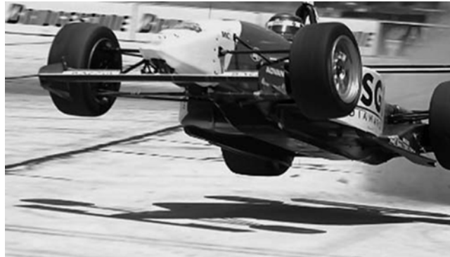
Figure 1.6 Positive lift at high speed can make a racecar airborne (unintentionally), emphasizing the need for a reliable downforce mechanism. Courtesy of Mark Page, Swift Engineering
