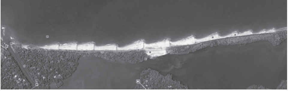
Fig. 1.2: A view of the coast of Paravoor, Kerala, showing the effect of groin field.
