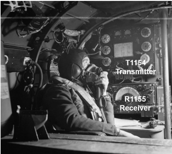
Figure 1.10 T1154/R1155 installation at the radio operators station in an Avro Lancaster, circa 1943.
