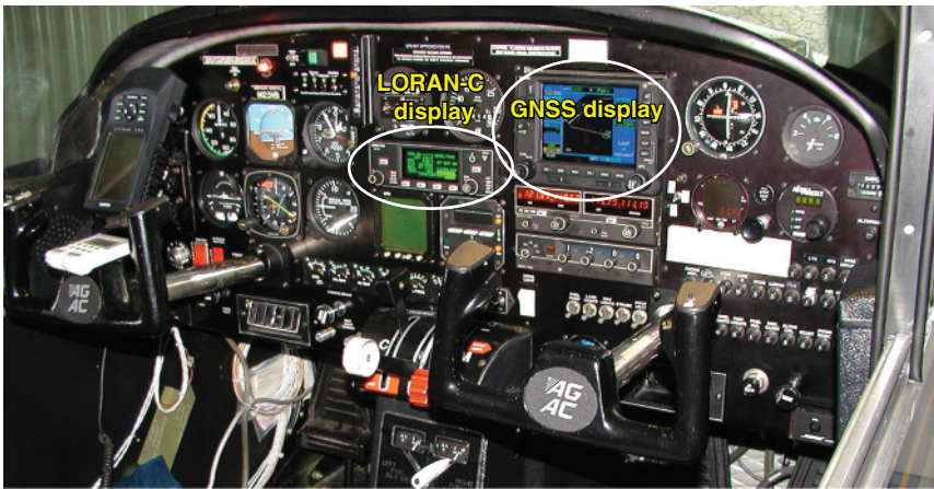
Figure 1.26 LORAN-C installed in a General Aviation aircraft (Grumman AA5) in the 1990s alongside a GNSS display. Source: Reproduced with permission of Rob Logan.
