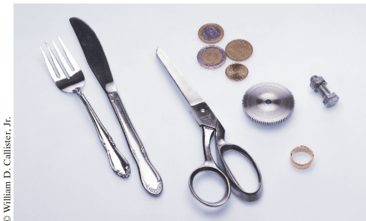
Figure 1.9 Familiar objects made of metals and metal alloys (from left to right): silverware (fork and knife), scissors, coins, a gear, a wedding ring, and a nut and bolt.
