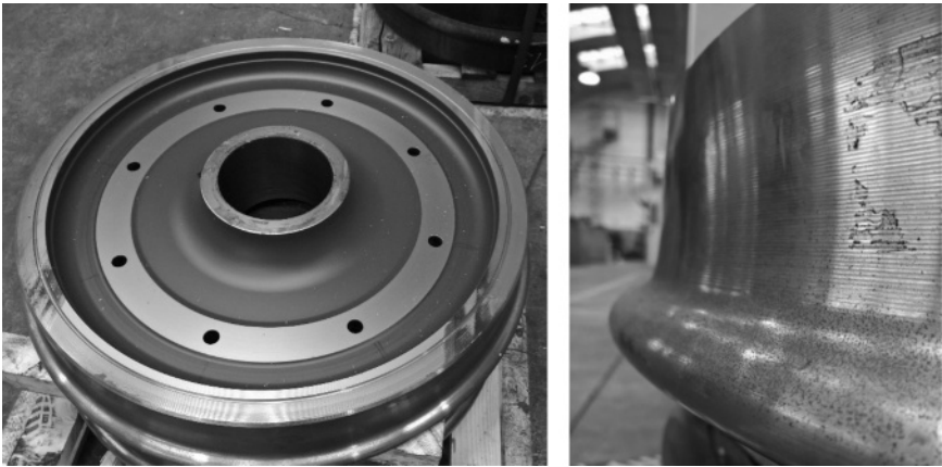
Figure 1.9 Steel wheels with rounded flange for railway and subway applications.
