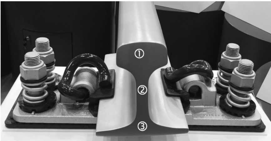
Figure 1.7 Section of a rail with linear mass of 60 kg/m (cross section = 7886 mm 2 ; moment of inertia J_x = 3055 \text{ cm}^4 ; moment of inertia J_y = 513 \text{ cm}^4 ) clamped on a sleeper: (1) head, (2) web, and (3) foot.
