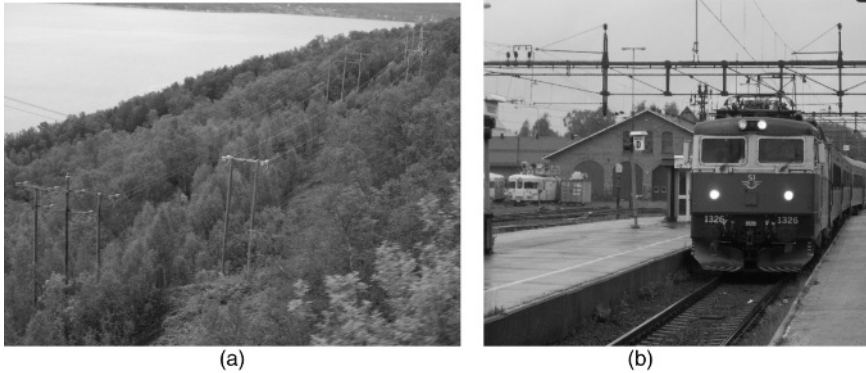
Figure 1.3 AC railway electrification system at railway frequency in Sweden: (a) primary lines and (b) railway line.
