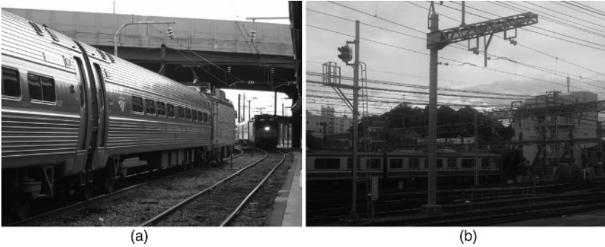
Figure 1.4 AC railway electrification system at mains frequency in (a) the United States and (b) Japan.
