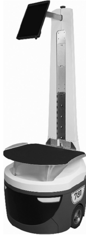
Figure 1.23 A mobile transport robot. Source: Reproduced with permission from Locus Robotics.
