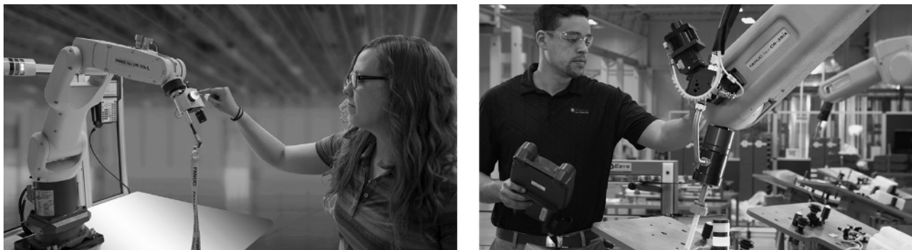
Figure 1.25 Collaborative robots are designed to detect the presence of humans around them and to collaborate with them. Source: Reproduced with permission from Fanuc America Corporation.
