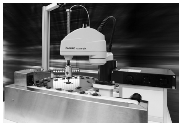
Figure 1.12 A robot engaged in sorting and inspection of manufactured parts. Source: Reproduced with permission from Fanuc America Corporation.
