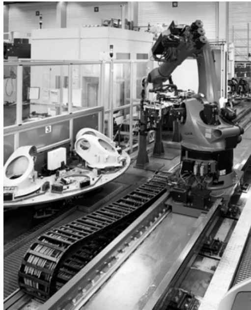
Figure 1.4 The robot can move along a track, adding a degree of freedom to the system. Source: Reproduced with permission from Kuka Robotics.
