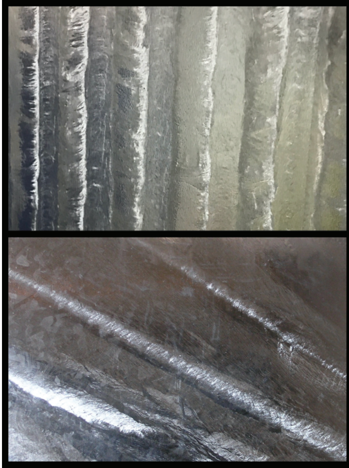
FIGURE 1.5 Zinc coating on steel using a controlled refinement of the cooling process.
