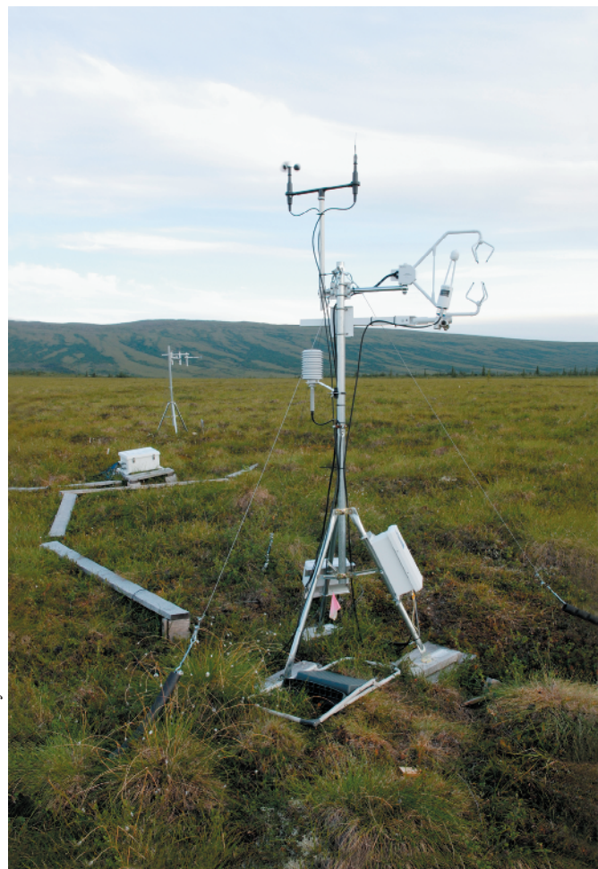
FIGURE 1.15 Climate change analysis. This equipment is part of a long-term project to explore the release of carbon dioxide (a greenhouse gas) from the melting tundra in Alaska.
