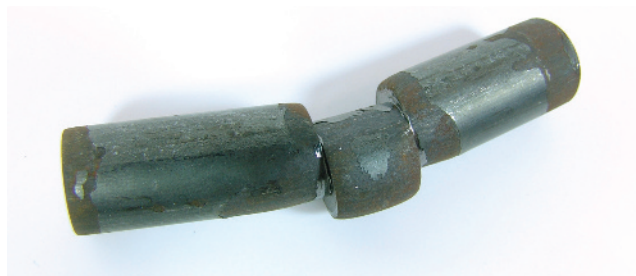
FIGURE 1.4 Double-shear failure in a pin specimen.
