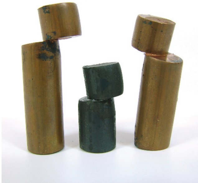
FIGURE 1.3 Single-shear failure in pin specimens.
