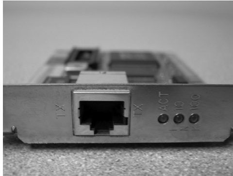
FIGURE 1.4 Photo of a typical network adapter
