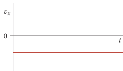
FIGURE 1.8.F A graph of x -velocity vs. time for an object traveling with a constant velocity to the left in the -x direction.
