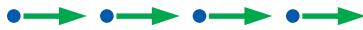
FIGURE 1.8.A An object moves to the right with constant velocity (uniform motion). Images of the object are shown at equal time intervals.
