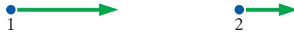
FIGURE 1.2.C Two successive positions of a particle (indicated by a dot), with arrows indicating the velocity of the particle at each location. The shorter arrow indicates that the speed of the particle at location 2 is less than its speed at location 1.
