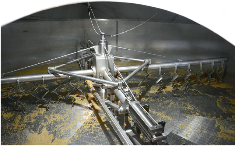
Figure 1.4 Lauter tun at Victory Brewing, Parkesburg, PA. Source: Photo by Naomi Hampson.
