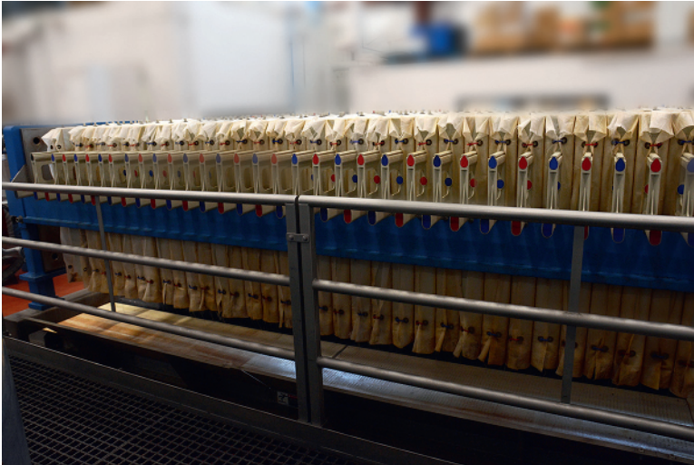
Figure 1.5 Mash filter at Bonesaw Brewing, Glassboro, NJ. Source: Photo by Naomi Hampson.
