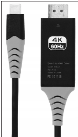
FIGURE 1-13: HDMI replaced the old VGA and DVI-D video adapters.
