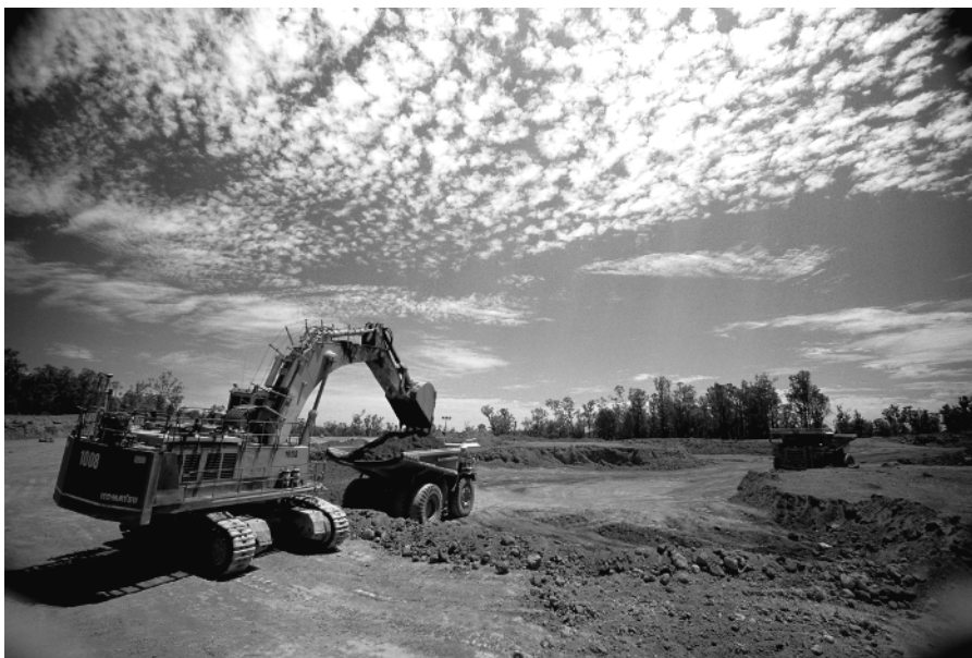
Figure 1.1 (Plate 1.1) Bauxite extraction at Huntley mine, southwestern Australia. On the Darling Plateau, bauxite is part of a mature soil profile developed over Archaean gneiss and granite. The area is covered by woodland (the jarrah, or Eucalyptus marginata forest). Mining depends on the availability of land and its social acceptance on rapid re-establishment of the native ecosystem. Reproduced by permission of Alcoa Inc.
